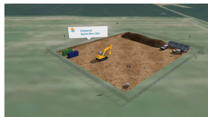
1. Site establishment including topsoil strip and store
