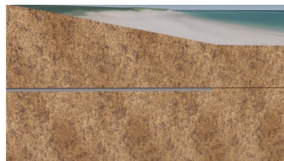
3. Pilot bore exits at reception pit
